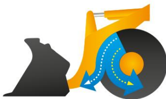
Normal pressure on the inching/brake pedal: speed reduction, more power in the service hydraulics.
