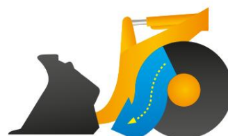
Maximum pressure on the inching/brake pedal: the wheel loader stops, maximum force for the hydraulic system.
