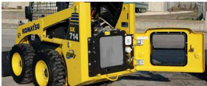
Rear Hood – Simple Inspection and Cleaning of Radiators
