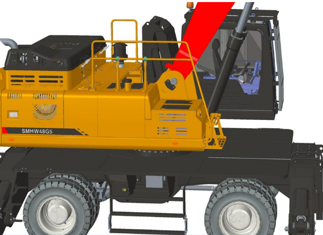
Handrails to engine bay, anti-slip surface, maintenance-panels on undercarriage
