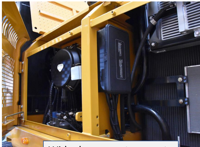
Wide doors grant access to radiators and filters
