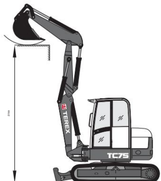
Fig. 2: Circular boom - dump height
